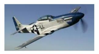
signed. The P-51 had a maximum speed of 440 miles per hour (almost 100 mph faster than the P-40) and a range of 1,650 miles (more than double the P-40). Technological innovation included an innovative laminar airflow wing, two speed automatic supercharger, automated fuel mixture controller, automated coolant temperature control, a 42,000 foot service ceiling, and a cost of \$50,000 in 1940 dollars.
